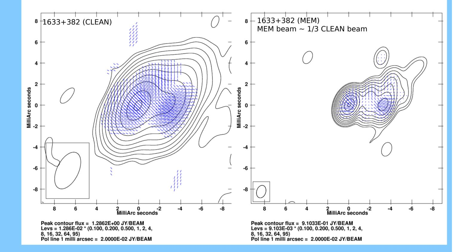
The CLEAN Fardaday rotation measure (RM) map constructed using VLBA data at 2-6cm provided evidence for a transverse RM gradient across the jet, possibly due to a helical B field [6]. The higher-resolution MEM RM map confirms this transverse RM structure, with a clear sign change in the RM from the Northern to the Southern part of the jet.
